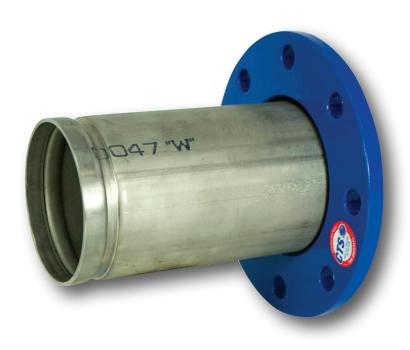
CTS HVAC-R now offer another innovative pipe line solution. The CTS Roll Grooved to Flanged Pipe Spool enables easy connection from a Flange to a component, with a roll groove end incorporated in the one integral unit. Designed for HVAC and civil water piping systems, the CTS RG Spool negates costly onsite fabrication.
